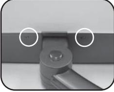
Remove the four (4) screws on the back of the unit using the included #2 Philips screw driver. (Only 2 screws are shown in photo).
