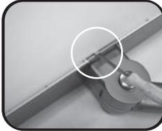
Gently remove the lens using a flathead (slot) screwdriver to raise the lens.
